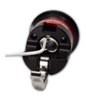
Loosen the two screws on the bottom plate spinner with a 2mm hex key.
