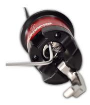
Place the assembled bottom plate spinner into the cavity and tighten the screws (torque: 0.5Nm - finger tight).
